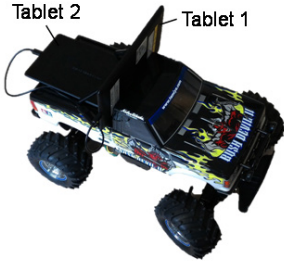
Fig. 9 Prototype UV controlled via LTE networks.
